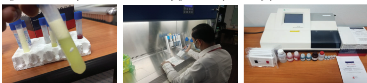
Fig 5: Ingenasa ELISA kit and ELISA Microplate Reader Model Teco Diagnostics Register Establishment Number 1832216 at O.D (450nm)
