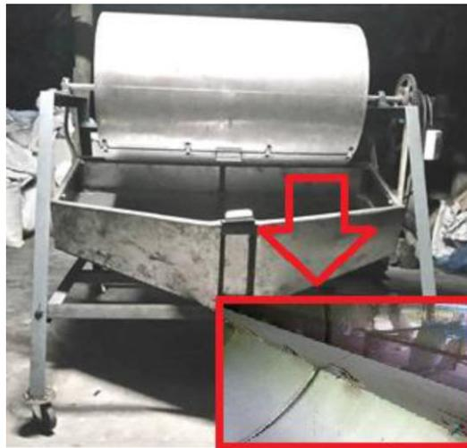
**Fig. 4 The developed rotating rice grain dryer prototype**
