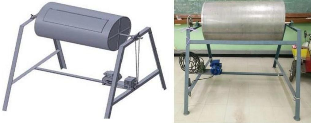
**Fig. 1 The original rotating rice grain dryer prototype**
