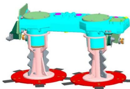
**Fig. 2 Base cutter blade (Ma et al., 2014)**
