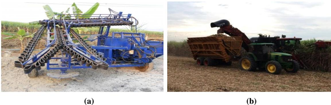
**Fig. 1 (a) The whole stick and (b) the chopper sugarcane harvesters (Opanukul et al., 2012)**
