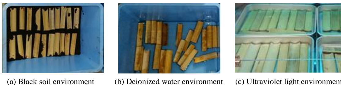
Fig. 2 Bamboo specimens with/without creosote oil treatment in different environments
