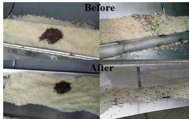
Fig. 5 Rice distributions in 30 minutes of the prototype operation observed by dark grain distributions among the white grains
