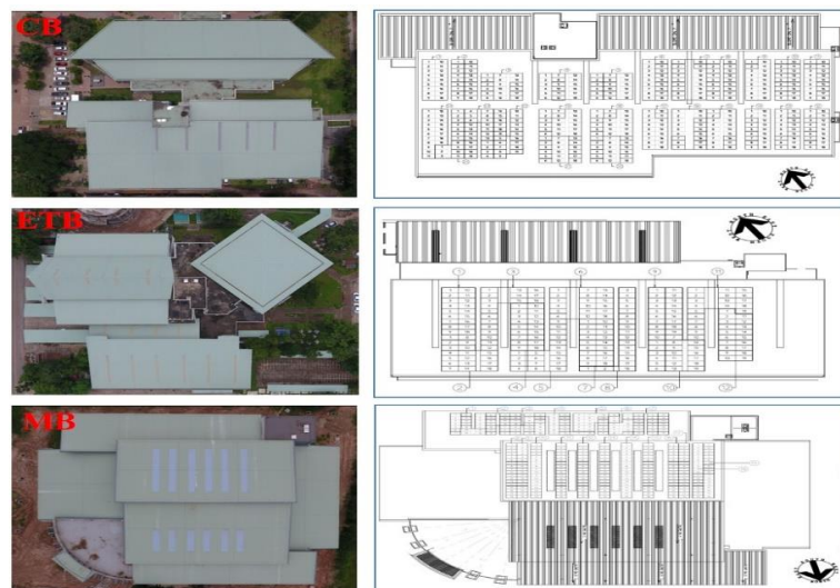
Fig. 2 Layout of solar PV rooftop system
