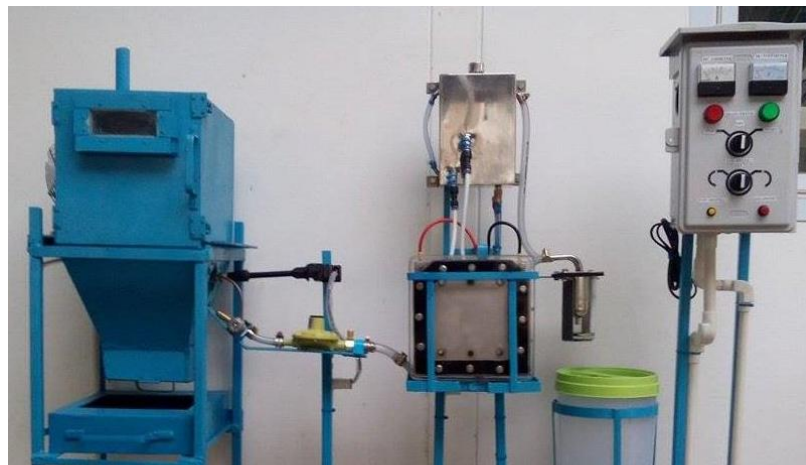
Fig. 3 The hydrogen gas incinerator plant with 3 sections
