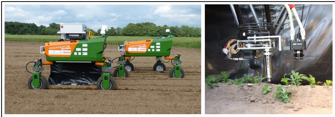
Fig. 1 Autonomous field robot platform “BoniRob” with and without Remote Farming.1 application for intra-row individual plant weed control (left). Manipulator and tube stamp actuator for single plant treatment (right)
