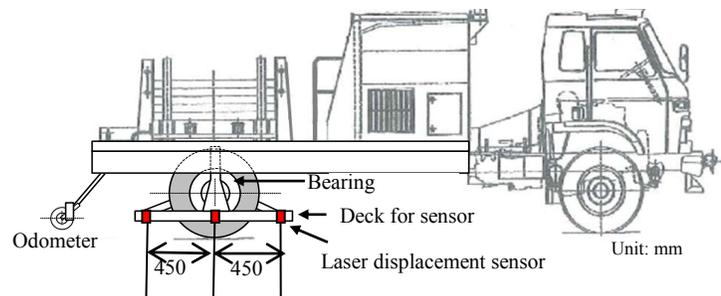
**Fig. 2 Sensor configuration**
