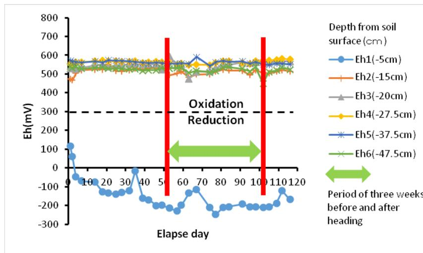
Fig.1 The temporal changes of Eh in the stratified paddy field model (O-70)
