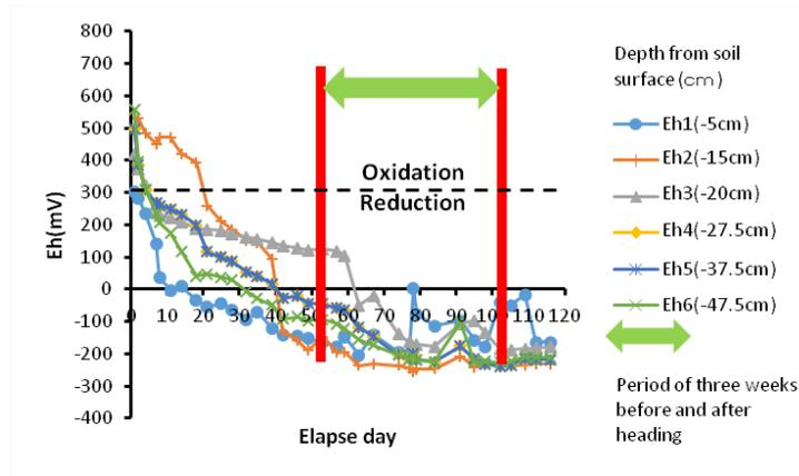
Fig.4 The temporal changes of Eh in the stratified paddy field model (C-250)
