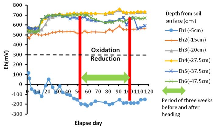
Fig.3 The temporal changes of Eh in the stratified paddy field model (O-250)
