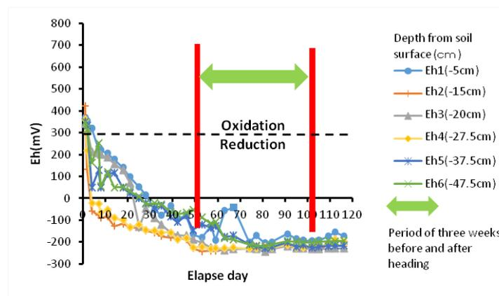
Fig.2 The temporal changes of Eh in the stratified paddy field model (C-70)
