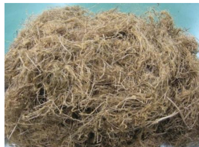
Photo 2 Bamboo fiber obtained by steam explosion
