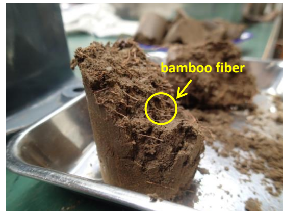
Photo 4 Shear failure surface of a specimen containing bamboo fiber
