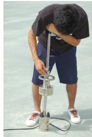
Fig. 6 PFWD testing in situ
