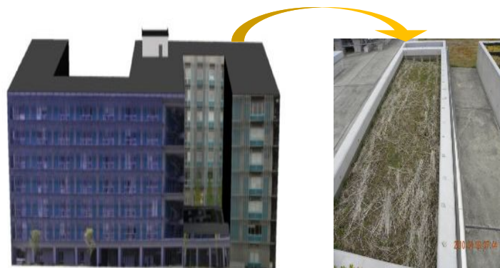
Fig.1 Lysimeter utilized in the study installed at the roof top
