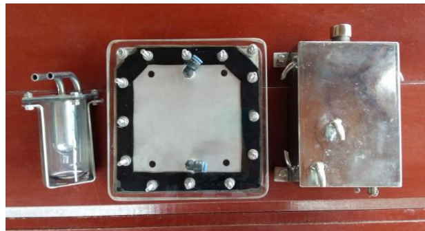
Fig. 1 Hydrogen gas production equipment
