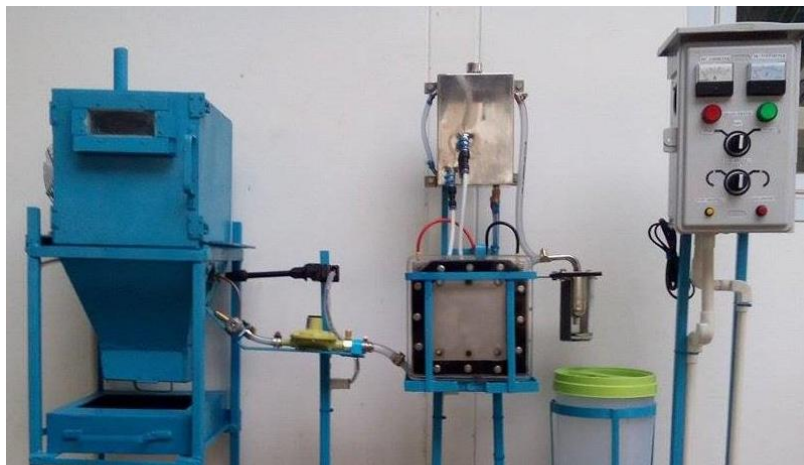
Fig. 3 The hydrogen gas incinerator plant with 3 sections
