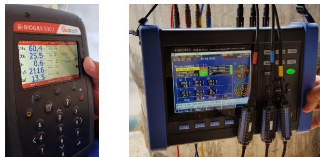
Fig. 1 Geotech biogas 5000 (left) and Hioki PW3365-20-01/5000 power logger (right)
