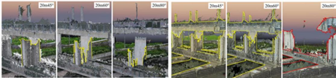
**Fig. 4 3D point cloud model created from aerial images of water gate**
