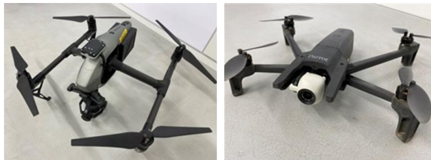
Fig. 2 Drones used in this study Inspire 2 (left) and ANAFI (right)
