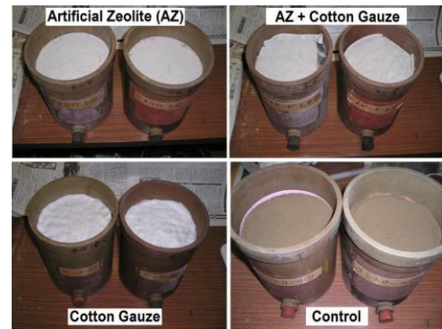
Fig. 5 Experiments of artificial zeolite and cotton gauze as salinity mitigators
