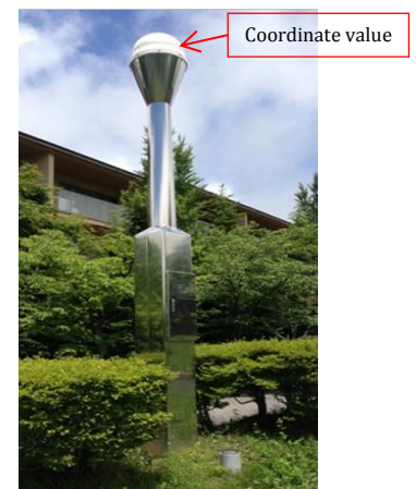
Fig. 3 GNSS-based control station No.950269
