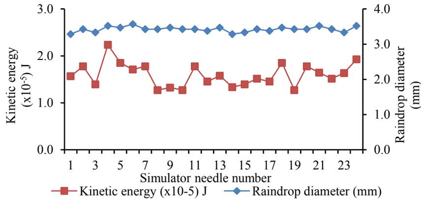
**Fig. 3 Kinetic Energy and raindrop diameter**
